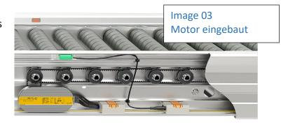
Control boxes, cables, sensors, etc. can be installed in the Avancon ZPC conveyor system very easily - and without tools - by simply pressing them onto the ASi cables at any point. This is because they lie parallel in the preformed ribs of the aluminum profiles. Eventual maintenance is very easy and fast.
