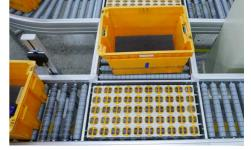
A convincing aspect was the safety of the Avancon system for human contact with the conveyors. A finger protection for each driven conveyor-roller doesn't exist anymore. Here is everything protected inside the conveyor frame – including the drive system and the control system. Nothing sticks out – not even a screw-head. Now the operators are freely working around the Avancon conveyors. The whole conveyor lines are
